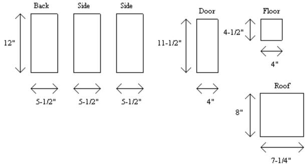
The back is nailed to the two sides. The roof is nailed on top of the back and the two sides. The sides are then nailed to the floor. The door is nailed to the two sides so it pivots from the top, and is held in place at the bottom by a latch.
